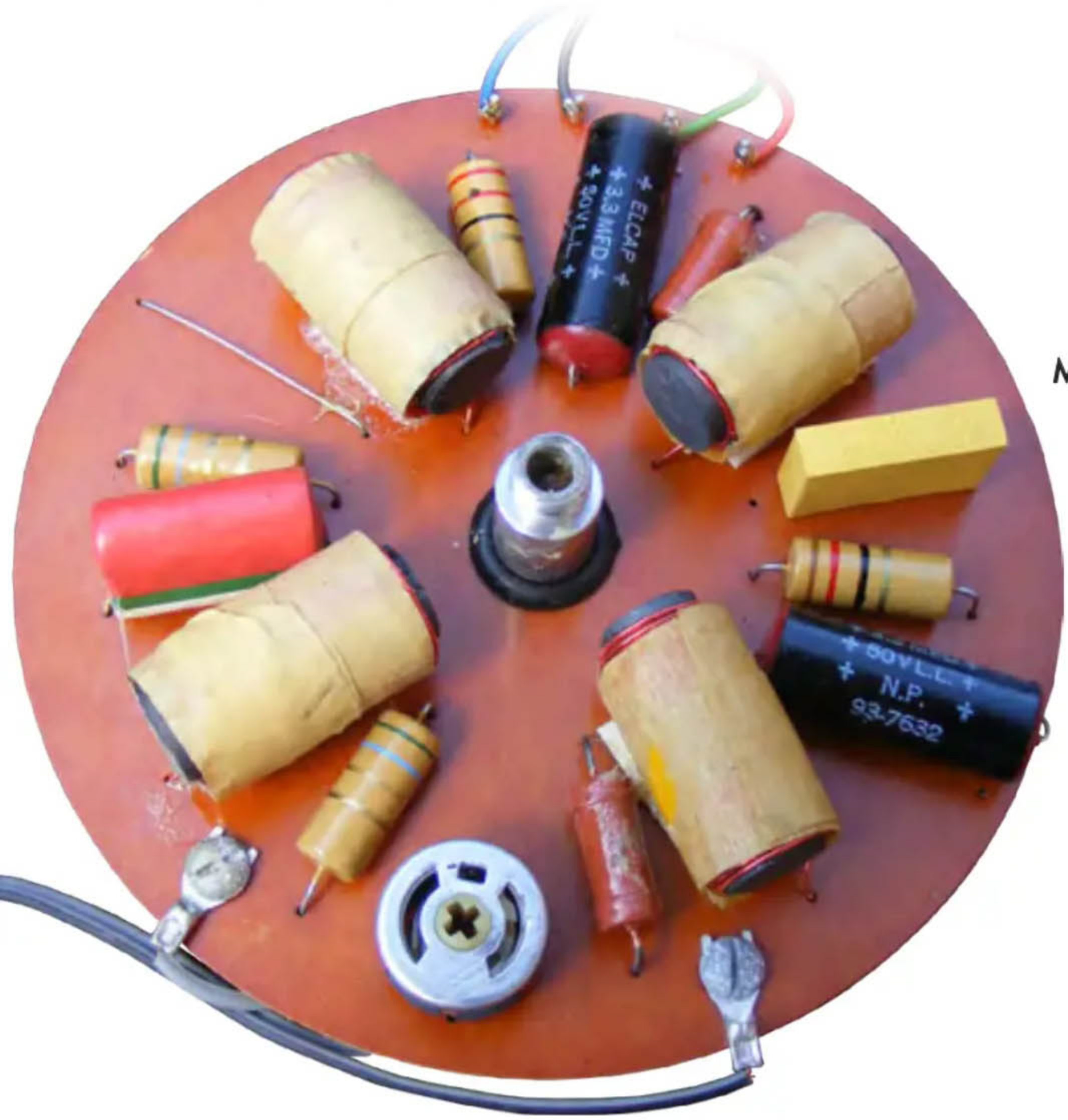
Fig.12: sometimes, low-loss bipolar electrolytics like 3.3µF Callins Elcaps are used in crossovers, such as this one from a JR149.
