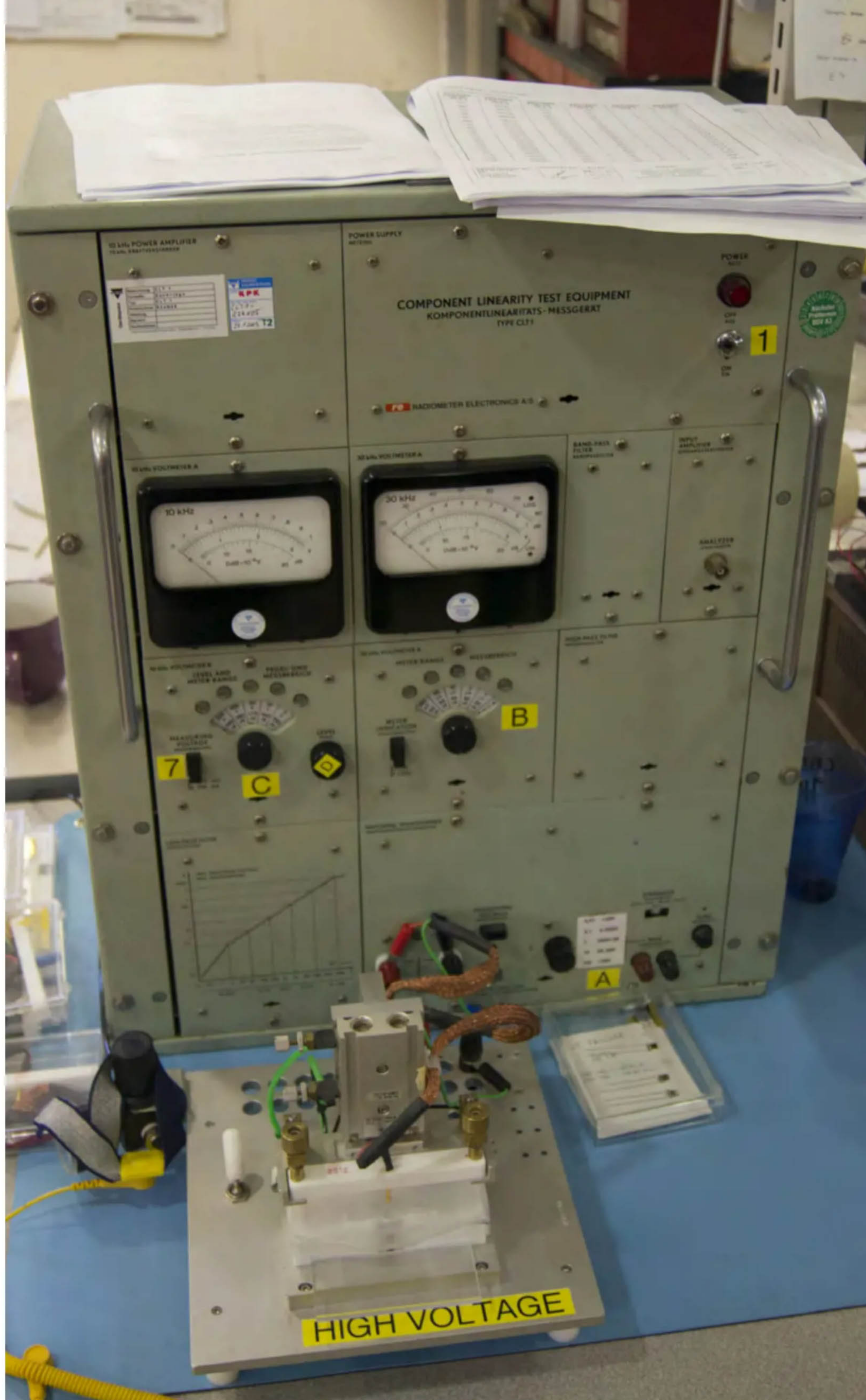
Fig.2: a component linearity tester at Charcroft's capacitor and resistor plant in Wales. It screens for bad contacts, which cause distortion.
