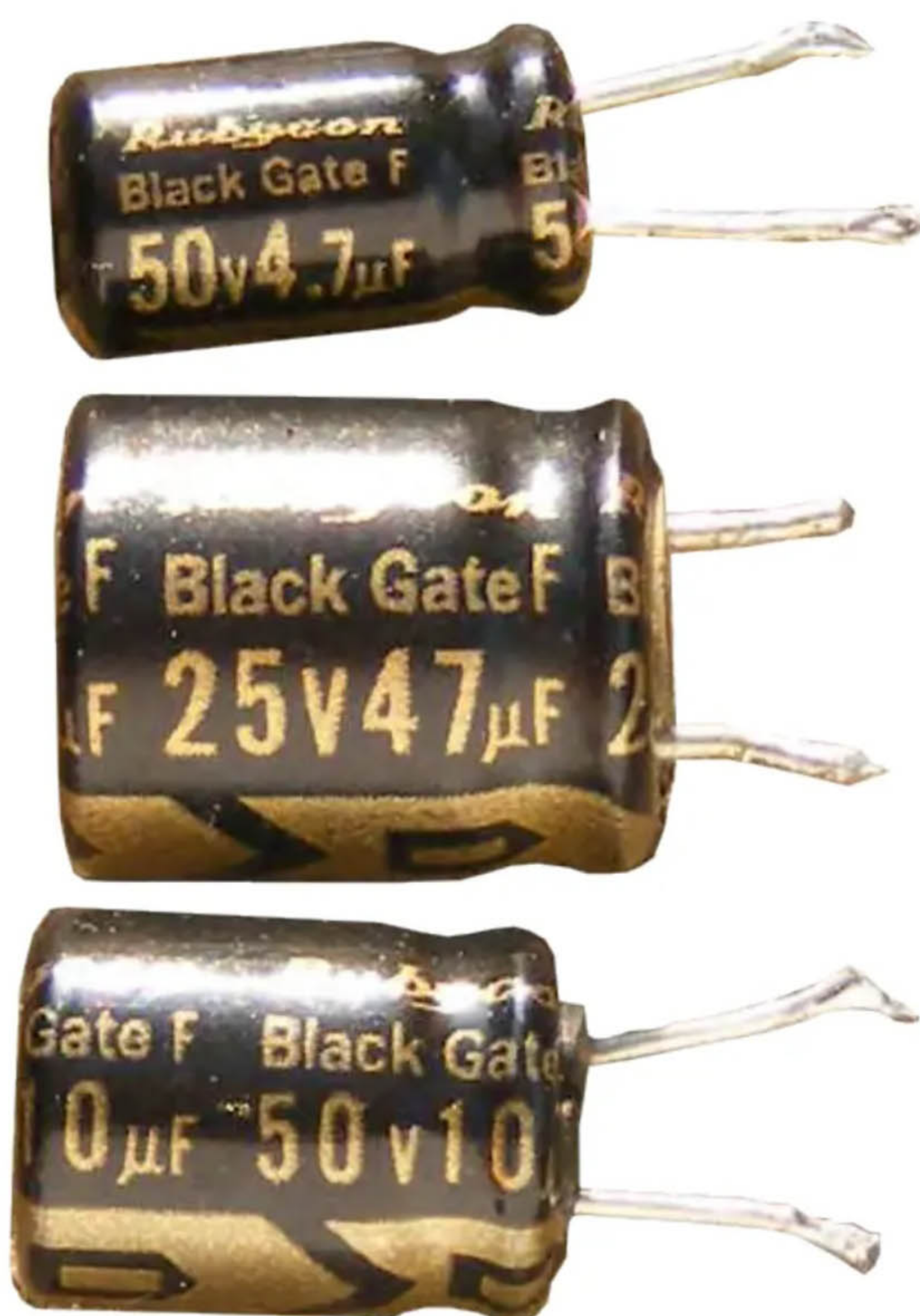
Fig.8: special Black Gate electrolytic capacitors for audio use by Rubycon. They are so expensive that I always reuse them if their ESR is okay.
